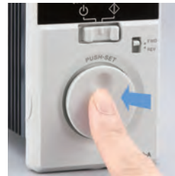
Pushing the dial sets the speed.
