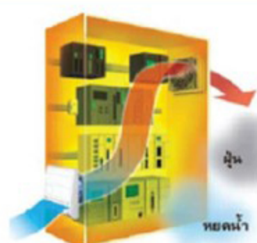
Cooling fan by Control Cabinet
